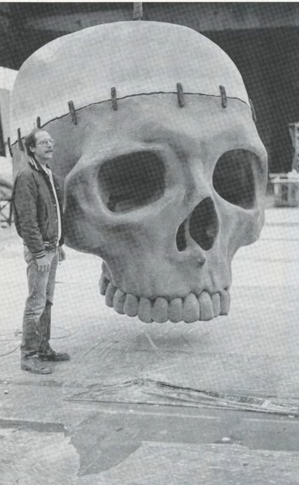
Jay Kotcher, Company head scenic artist, pauses by a remarkable object that emerged out of his department. The skull, which will dominate the Klingsor scene of Parsifal , was first sculpted out of styrofoam, then coated with fiberglass. After the styrofoam was removed, the resulting shape was finished, outfitted with "stitches" and readied for its translucent debut on stage.
