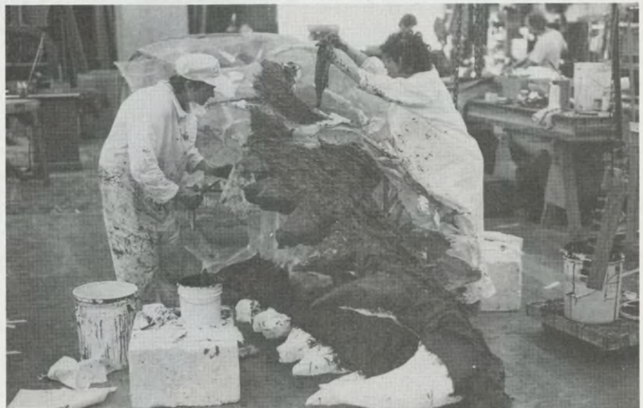
The dragon, taking shape in the San Francisco Opera Scene Shop: (above) the skull is being covered by a wire screen, (below) Elizabeth Jennings and Donna Mossholder are engaged in "ragging"—pieces of gauze dipped in colored glue are applied to the basic structure and the styrofoam teeth.
